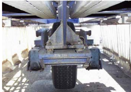
Figure 3. Federal Highway Administration's Pavement Testing Facility Showing Both Accelerated Loading Machines and Close-Up of Super-Single Loading Wheel Tire
