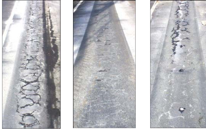
FIGURE. 11 Representative Photographs of Three PTF Lanes [Left] Lane 2 (Control) after 100,000 loadings; [Middle] Lane 4 (SBS) after 300,000 loadings; and [Right] Lane 5 (CR-TB) after 100,000 loadings.
